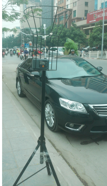
Figure 1: Taking VOCs samples in near road in Hanoi
