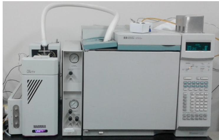
Figure 2: GC-FID in Kyoto University to analyze VOCs
