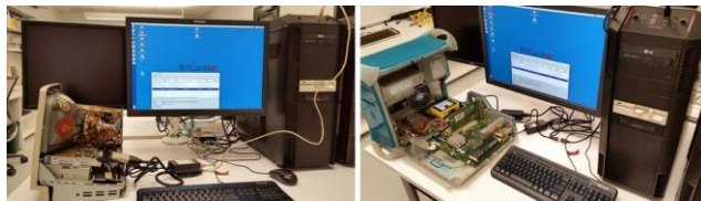
Figure 1: Digital forensics software and hardware being used to capture the content of hard drives from original computers.
