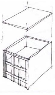
Strength and stiff moment-resisting or braced frame is designed for soft front wall
