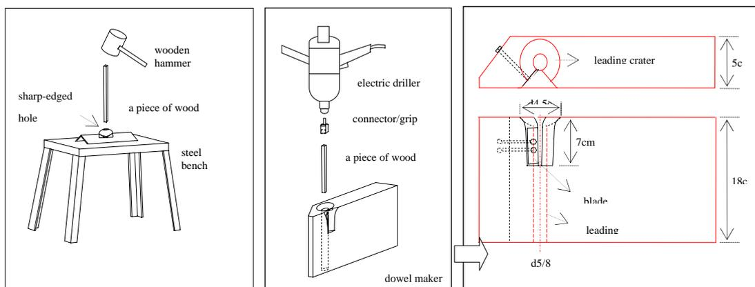
**Fig. 6** Sharp-hole dowel maker    **Fig. 7 and 8** Pencil-sharpener dowel maker and details
