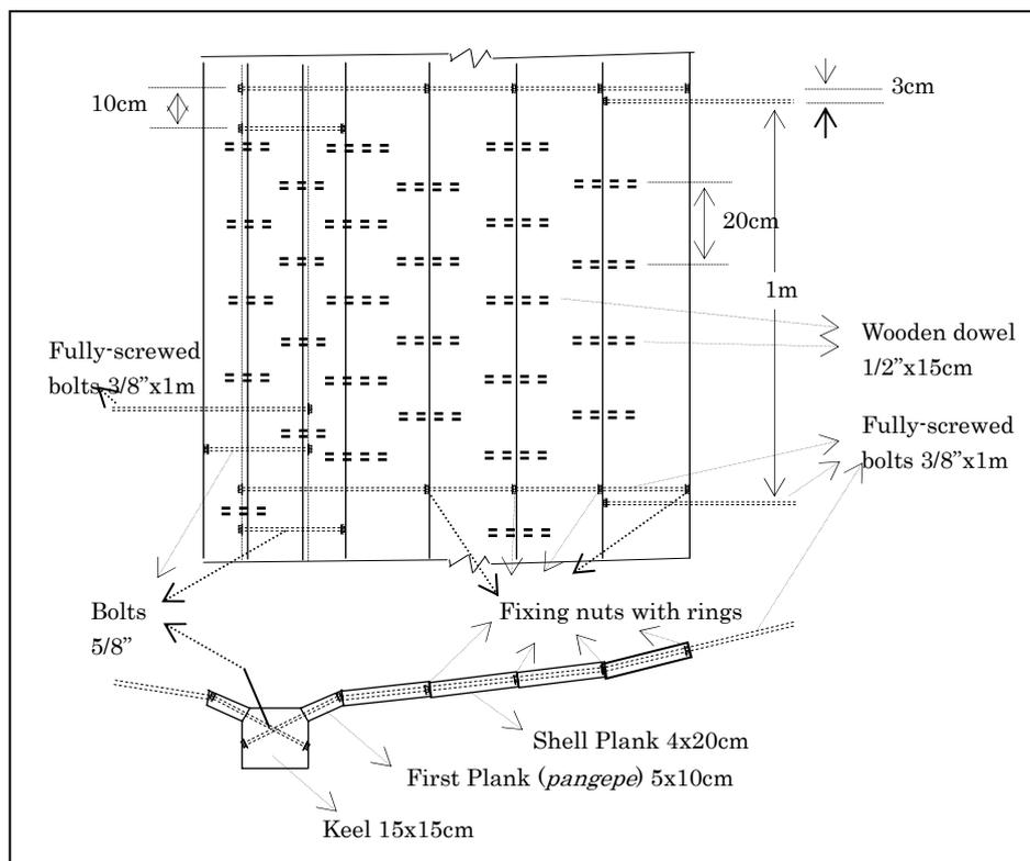
**Fig. 5** The fishbone plank-fastening system
