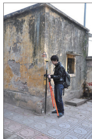
DGPS基準点測量調査 Base point measurement with DGPS
