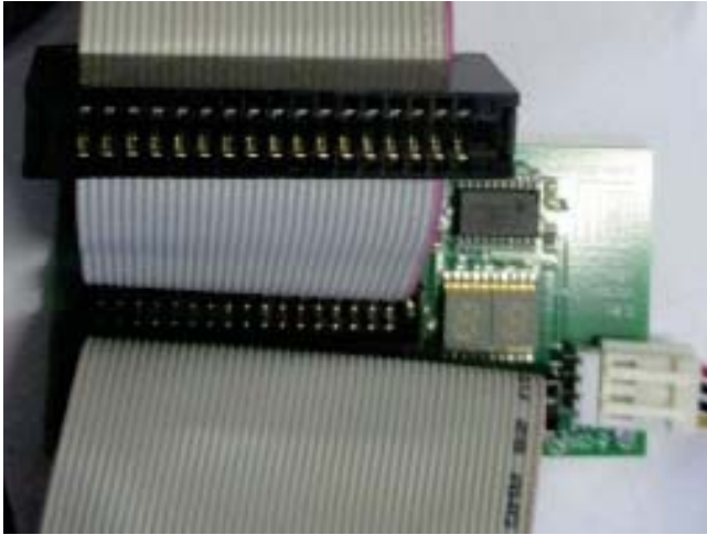
Figure 3: Electrically adapting the drive and providing a track readout
